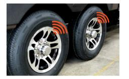
Sensors update pressure and temperature several times each minute while your RV is moving and check every 15 minutes while parked. Notifications sent any time the tyres inflate, deflate or in the case of a blowout
