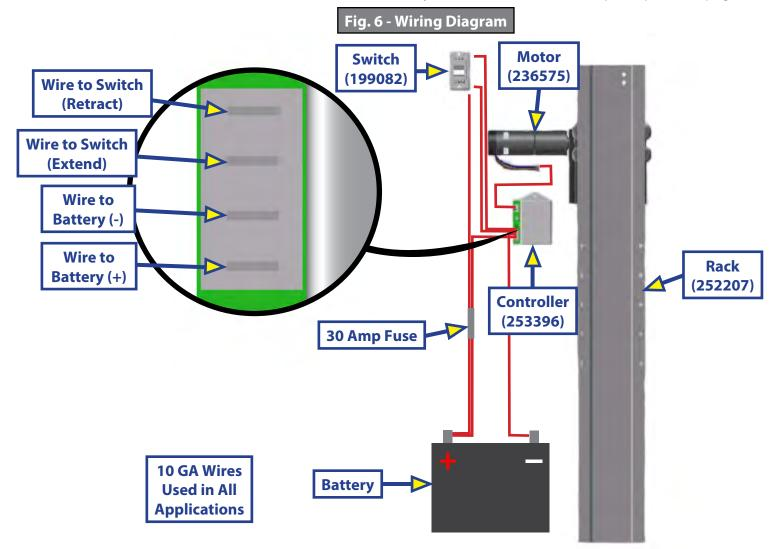
**NOTE:** Wire harness to battery and switch is customer supplied. Harness wires must be 10 gauge minimum. A 30 amp breaker should also be installed on the power lead between the battery and the controller.
