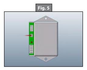
**NOTE:** To pull the TV and rack back out of the lift unit, press and hold the MODE button for 5 seconds. The RED light will illuminate and the GREEN light will flash. At the switch, push the switch UP and the lift will extend the rack so it can be removed from the system. To re-install, see steps on previous page.
