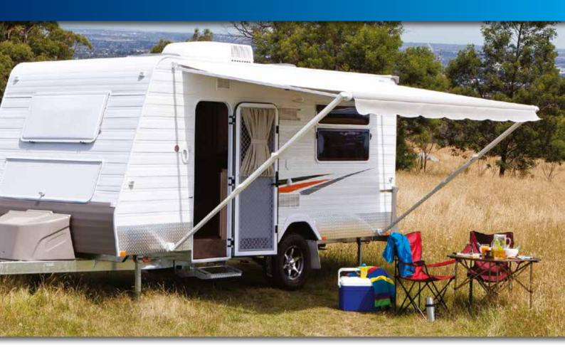
The Carefree Fiesta is a manual, spring loaded, rollout awning with vinyl weathergard. Its multi-layer vinyl canopy is one of the best awning fabrics available so it is constructed to last!
