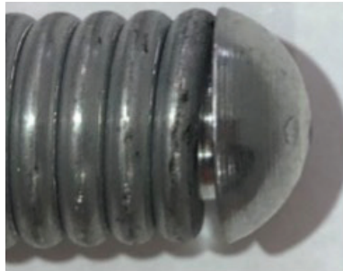
Riveted end at the roof of camper.
