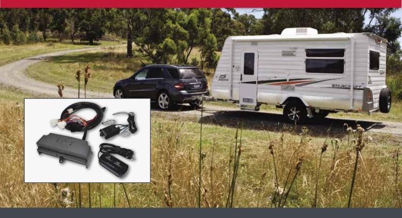
A 'break-away' system is compulsory on all trailers over 2,000kg GTM. Each state/ territory has their own rules regarding their towing legalities. For example, all trailers registered in NSW are required to have a brake battery monitor fitted. This brake battery monitor needs to be visible from the driver's seat. Coast recommends contacting your local roads and traffic authority regarding your state's towing legalities.
